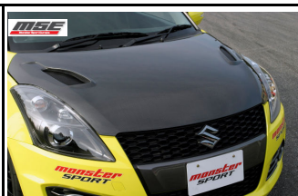
Carbon Front Hood 8JQB10 95,000JPY Material: C.F.R.P Weight: 5.8kg (STD 9.4kg)
