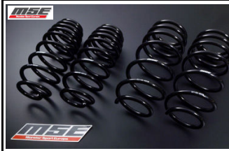
Lowering Spring Set 520500-4850M 28,000JPY Spring Rate Fr: 2.9kgf/mm Rr: 3.5kgf/mm Ride height: -25~-30mm
