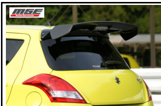
Carbon GT Rear Wing 8JQW20 85,000JPY Material: C.F.R.P Weight: 3kg
